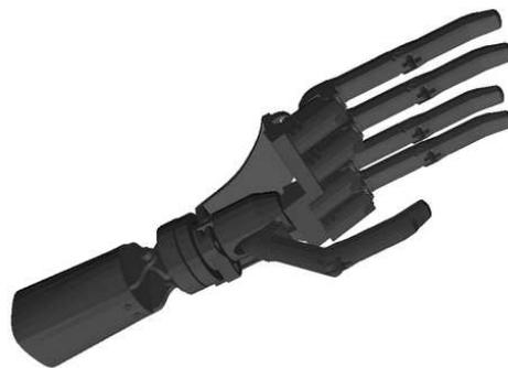
**Fig. 1.** 3D Hand Prosthesis Model.
