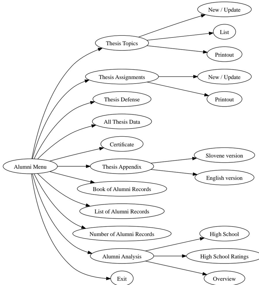
**Fig. 4.** The use case diagram for theses and alumni records: internal nodes represent (sub)-menus, leaves represent the main operations.
