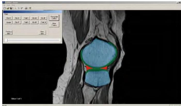
**Fig. 4.** Segmentation of the knee model from MRI slices. Sagittal view MRI of the left knee. The bone geometry, cartilages and meniscuses are digitized for 3D finite element model
