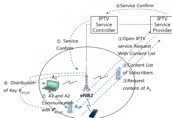
**Fig. 8.** Pairwise key establishment between devices for open IPTV in the same cell
