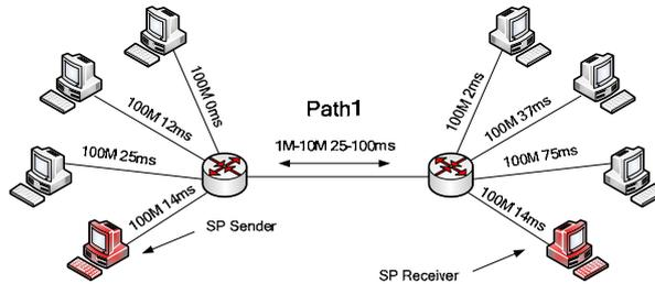
Fig. 6 Topology for single path transport
