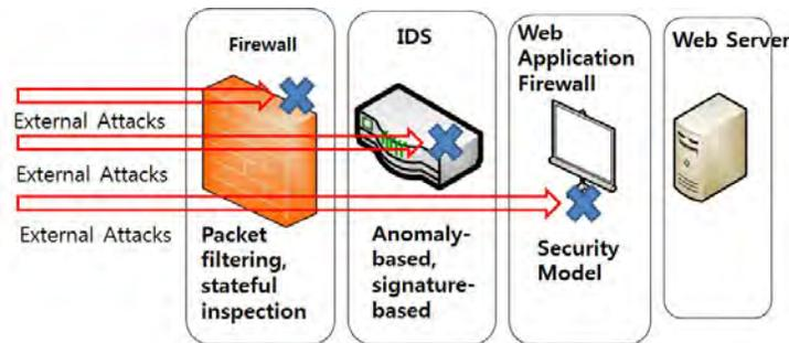
**Fig. 1.** Traditional Layered Security System for Web server
