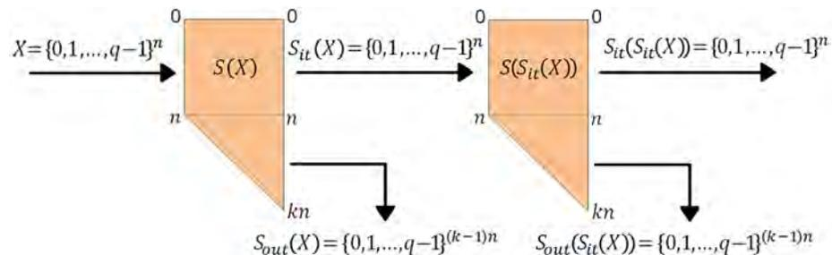
**Fig. 1.** Generating keystream of QUAD
