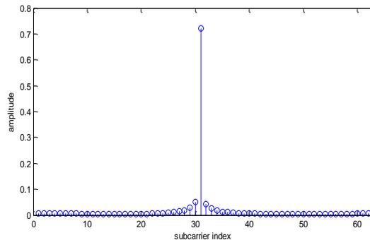
**Fig. 7.** The ICI amplitude for the desired signal at subcarrier 30
