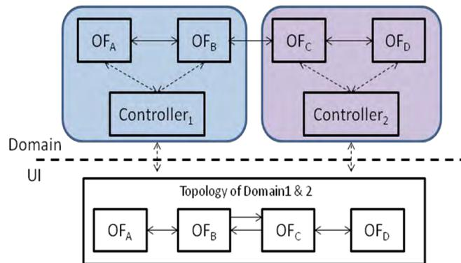
**Fig. 6.** Inter-domain information after applying proposed mechanism.
