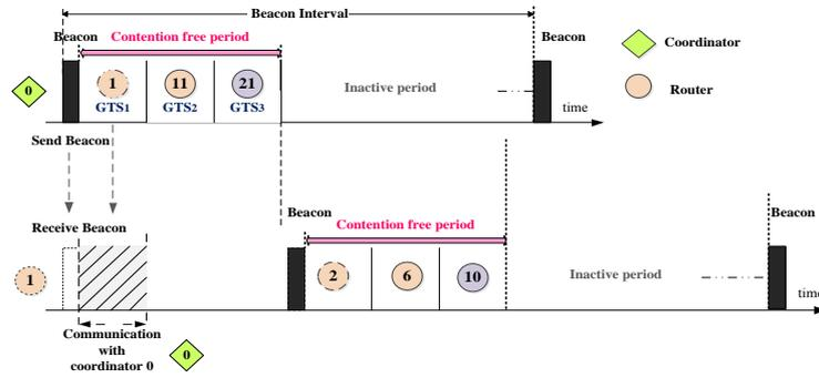
Fig. 2 The relation between coordinator and child device
