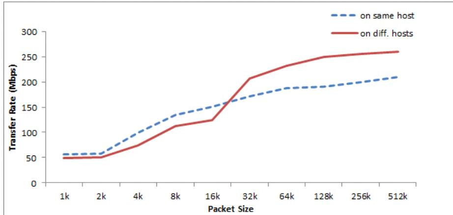
Fig. 11. Throughput of different VM assignment approaches.
