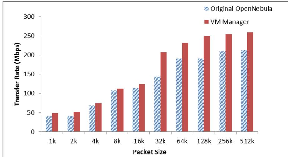
Fig. 13. Throughput with VMs on the different hosts
