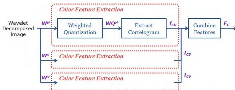
**Fig. 3.** Procedure for Weighted Wavelet Spatial Color Extraction.
