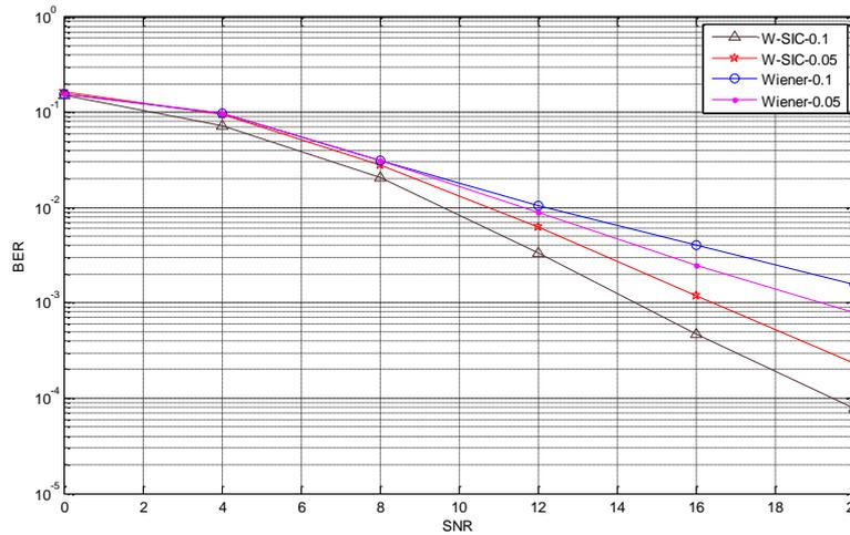
Fig. 10. BER versus SNR for different  $f_d T_s$
