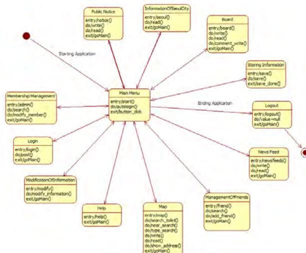
Fig. 8. The proposed state diagram
