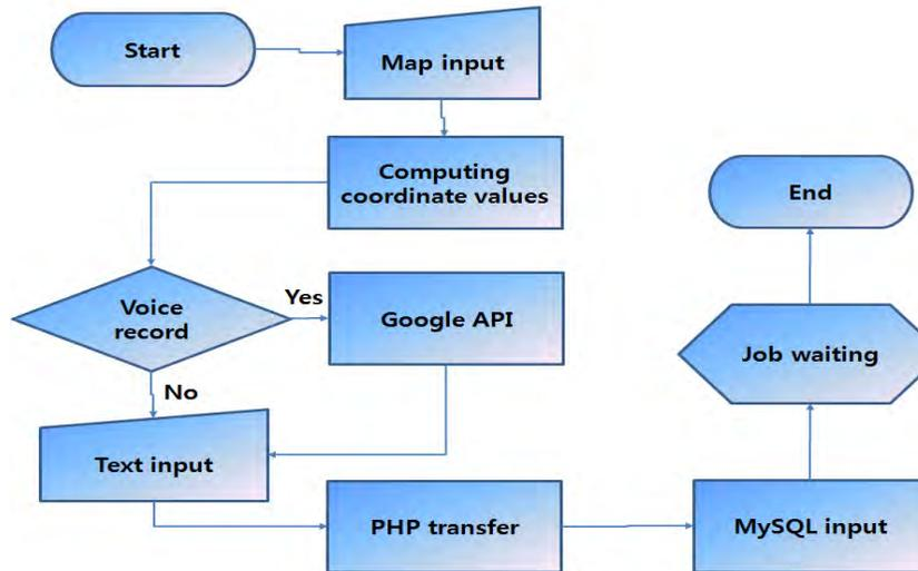
Fig. 11. A flowchart for inserting coordinate values
