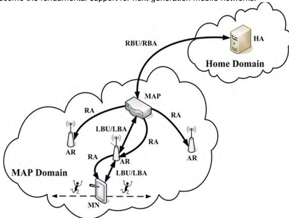
Fig 1 HMIPv6 network
