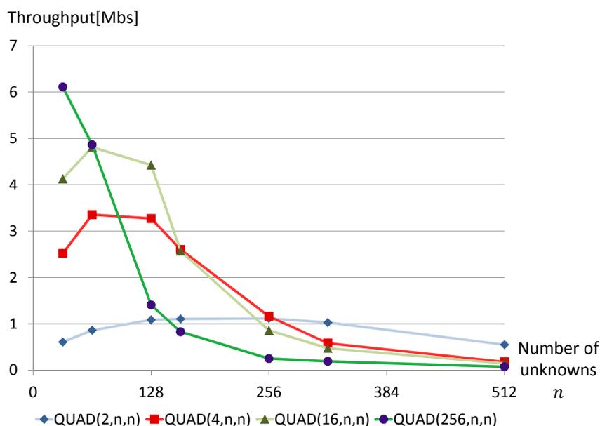
**Fig. 6.** Throughputs of QUAD implementations over  $GF(2^t)$  ( $t = 1, 2, 4, 8$ )
