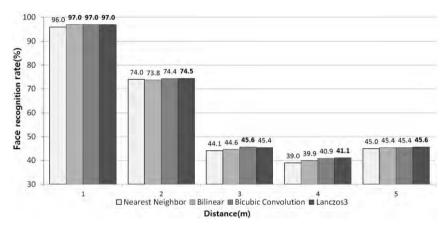
Fig. 6. Face recognition rate of CASE 1 according to interpolations
