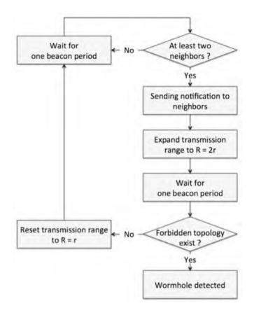
Fig. 5. Wormhole Detection Process
