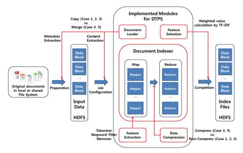
Fig. 5. The implemented modules of DTPS and control flow for each different experiment
