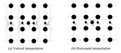
Fig. 2. Bicubic convolution interpolation
