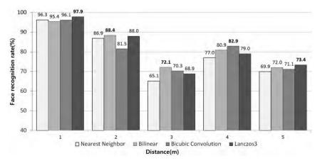
Fig. 7. Face recognition rate of CASE 2 according to interpolations
