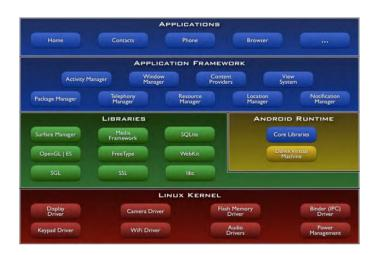
Fig. 1. Android system architecture.
