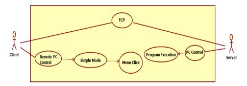
(a) Use case diagram of simple mode
