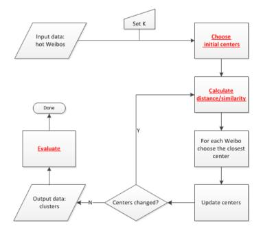
Fig. 1. The flow chart of K-means++ used in this paper
