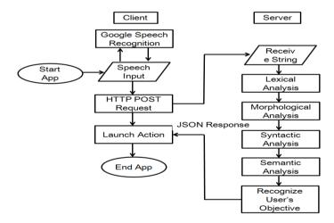
Fig. 2. Data flow diagram of speech recognition.
