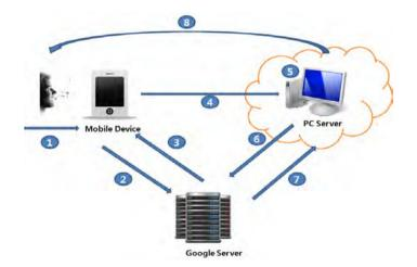
Fig. 4. Command transmission methods among a mobile device, a Google server, and a personal computer server.
