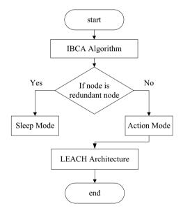
Fig. 2. The flow chart of LEACH architecture with IBCA
