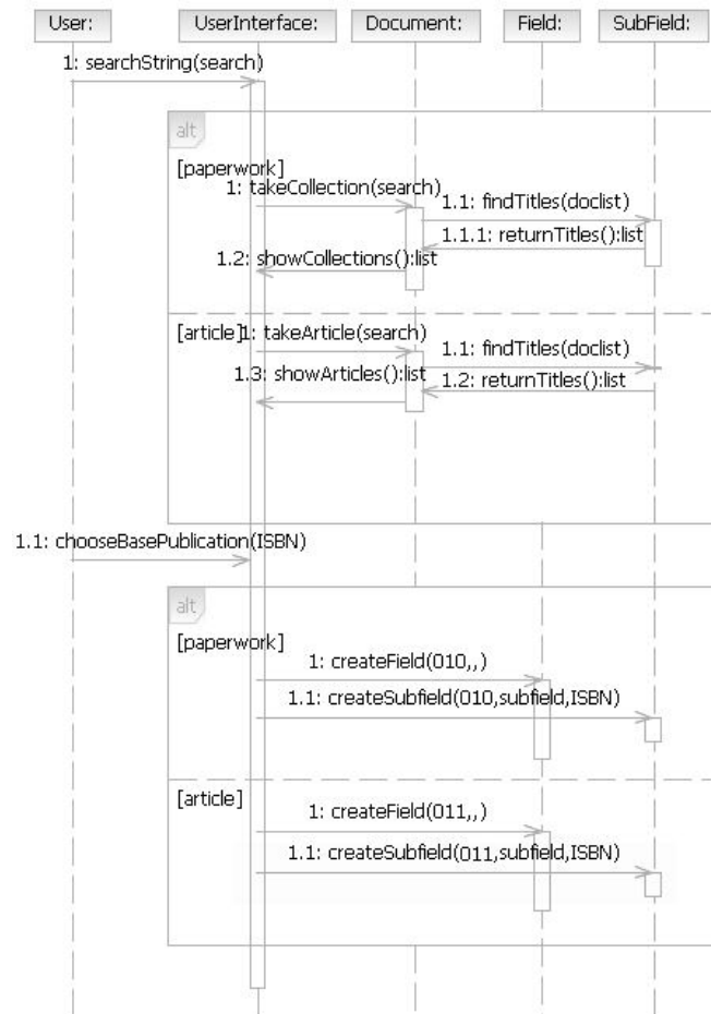
Fig. 3.8. Sequence diagram for the use case Base publication
