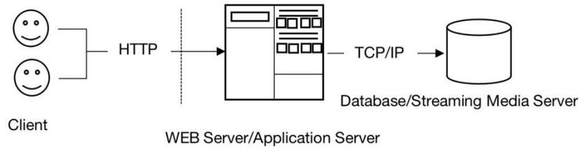
**Fig. 2.** System architecture
