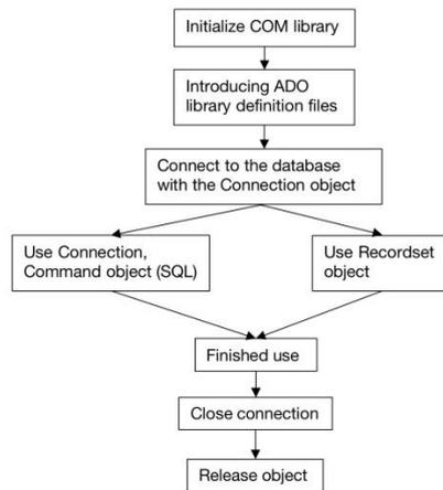
**Fig. 3.** System database development process
