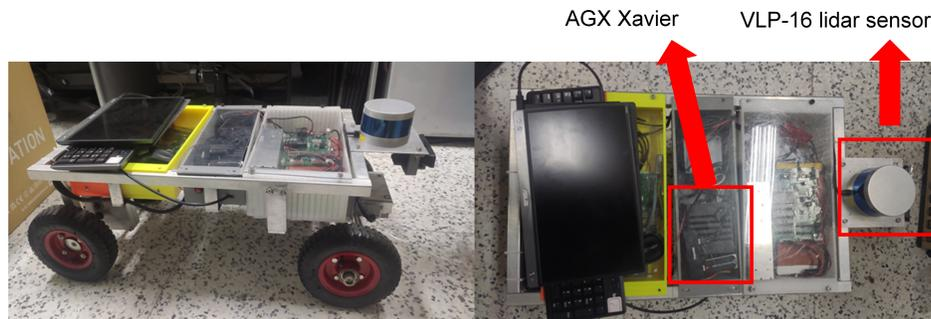
Fig. 2. Designed autonomous Ackerman robot
