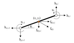
Fig. 2. The forces and torques acting on each link of the snake robot
