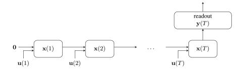
**Fig. 2.** Unfolding in time of the Gated ESN and Gated ESN RZ architecture for a sequence of length T. Each state  $\mathbf{x}(t)$  is computed by the recurrent cell illustrated in Fig. 1. Since in this work we are concerned with the classification of a sequence given the last time step, we only show that configuration.
