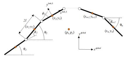
**Fig. 1.** *n* links snake robot diagram
