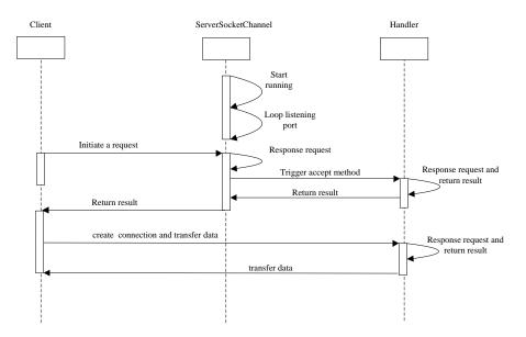
Fig. 5. The process of asynchronous IO
