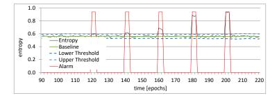
Fig. 8. The Shannon entropy and the N1-1N model - the source IP address feature aggregated by the destination port (S[d]).
