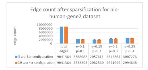
**Fig. 9.** The degree of sparsification, i.e. the remaining edge counts after the calculation, for the bio-human-gene2 dataset. The results are shown for some parameter combinations and compared to the edge count of the dataset before sparsification
