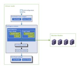
**Fig. 4.** An overview of the architecture. It shows what parts of the contingency analysis are performed on the driver node and which are distributed across a collection of worker nodes
