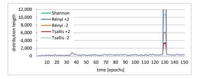
Fig. 5. The length of the d[S.D] feature distribution with spoofed traffic.
