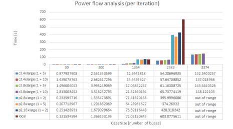
Fig. 5. The performance results of the power flow analysis, scaled to per-iteration values
