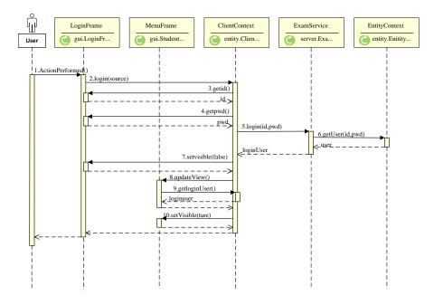
Fig. 6. The process of login function
