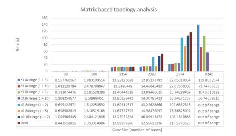
Fig. 6. The performance results of the matrix based topology analysis
