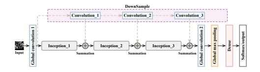
**Fig. 2.** RICNN network model architecture. Its input is a  $16 \times 16$  grayscale matrix. The main structure of RICNN is three residual blocks, each of which consists of an Inception unit and a direct mapping. In addition, there are several global network layers to increase and reduce the dimension of the feature maps, and finally the model prediction results are output through the Softmax layer
