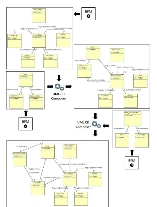
Fig. 12. Illustration of incremental CDM composition based on sample source set of BPMN models
