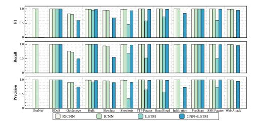
**Fig. 8.** Comparison of evaluation indicators between the proposed models and the RNN models for imbalanced abnormal traffic (header)
