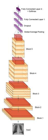
Fig. 2. The adapted VGG19 convolutional neural network architecture.
