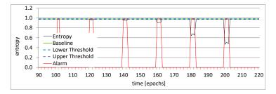
Fig. 7. The Shannon entropy and the N1-1N model - the flow count feature aggregated by the source port (f[s]).
