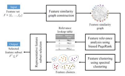
Fig. 3. Process flow of FS-SCPR
