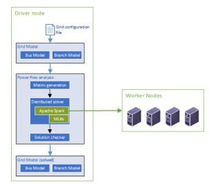
Fig. 1 An overview of the architecture. It shows what parts of the power flow analysis are performed on the driver node and which are distributed across a collection of worker nodes
