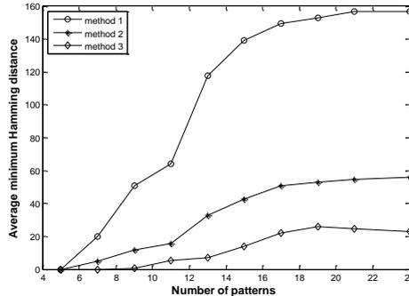
**Fig. 5.4.** Average minimum Hamming distance for the three frequency based kernel methods in respect to the size of the pattern space.
