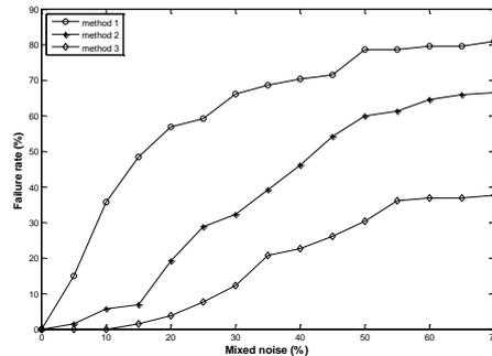
**Fig. 5.6.** Failure recall rates of the three frequency based kernel vector methods in respect to mixed noise percentage.
