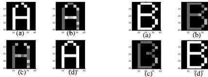
**Fig. 4.3.** Examples of perfect recall using the new kernel vectors and input vectors corrupted by the erosive noise described in section 3. (a) the corrupted vector used as input (b) the original kernel vector (c) non-perfect recall of the kernel vector by (2.5) (d) perfect recall of the pattern by (2.9)
