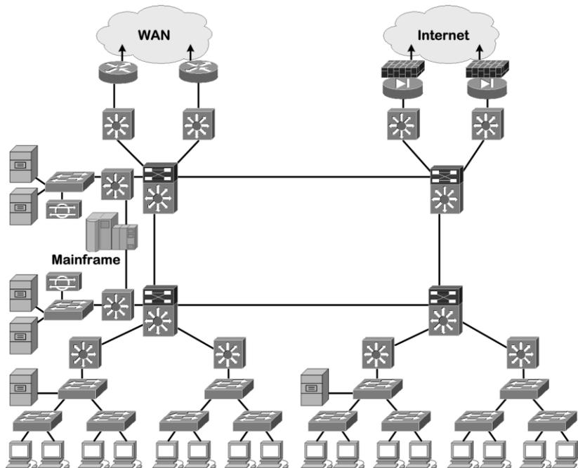
**Fig. 10.** A hierarchical scalable network design model
