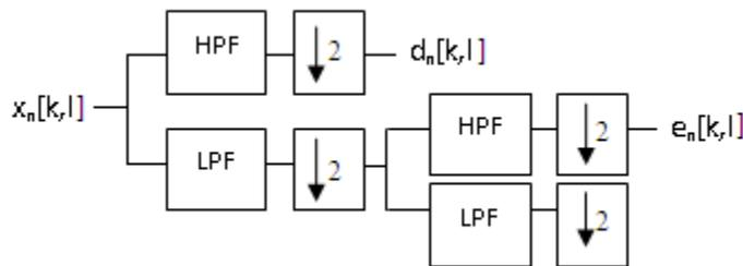
Fig. 7. A two-stage filter with HPF and LPF
