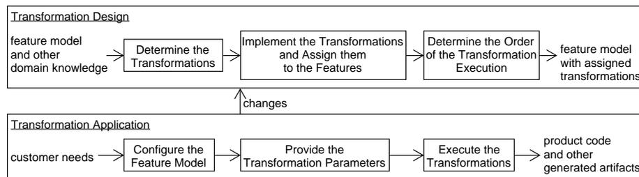
**Fig. 3.** The overall process.
