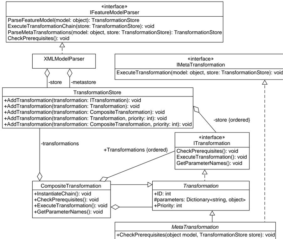
**Fig. 4.** The overall architecture.
