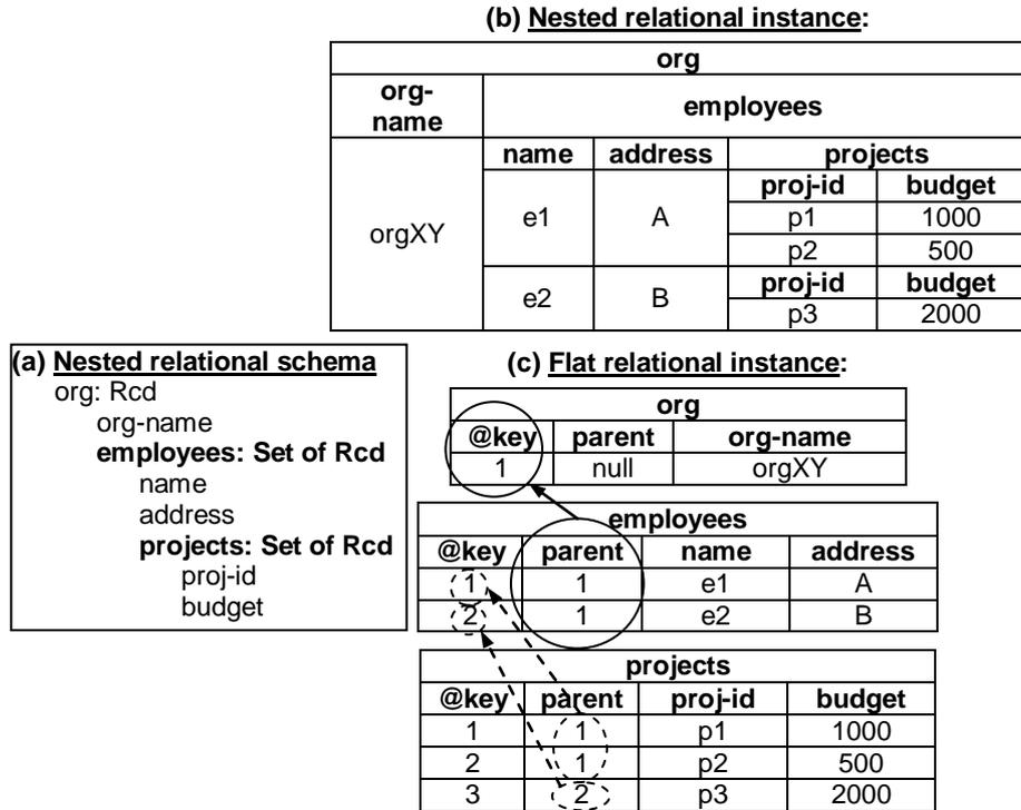
**Fig. 3.** A (a) nested relational schema, an (b) instance of this schema, and (c) the translation of the instance into flat relations
