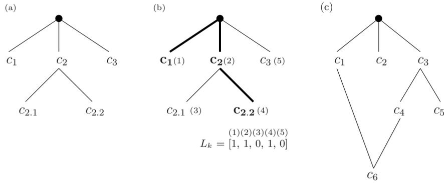
**Fig. 1.** Toy examples of hierarchies structured as a tree and a DAG. (a) Class label names contain information about the position in the hierarchy, e.g.,  $c_{2.1}$  is a subclass of  $c_2$ . (b) The set of classes  $S_1 = \{c_1, c_2, c_{2.2}\}$ , shown in bold in the hierarchy, represented as a vector ( $L_k$ ). (c) A class hierarchy structured as a DAG. The class  $c_6$  has two parents:  $c_1$  and  $c_4$ .
