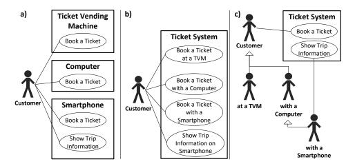
Fig. 2. Different workarounds to partially model the running example with standard UML use case diagrams: a) Depict every device type as a separate system, b) encode device type information within use cases, c) combine device type information with actor roles.
