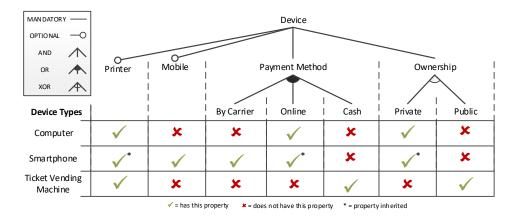
Fig. 10. Specification of device properties in terms of a feature diagrams (upper part) and assigning device properties to device types (lower part)
