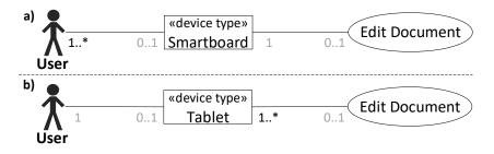
Fig. 4. Example for editing a document with multiple users: (a) All users collaborate on a smartboard and there is only one smartboard per use case instance, (b) multiple tablets are used to collaborate and there is only a single user per tablet.
