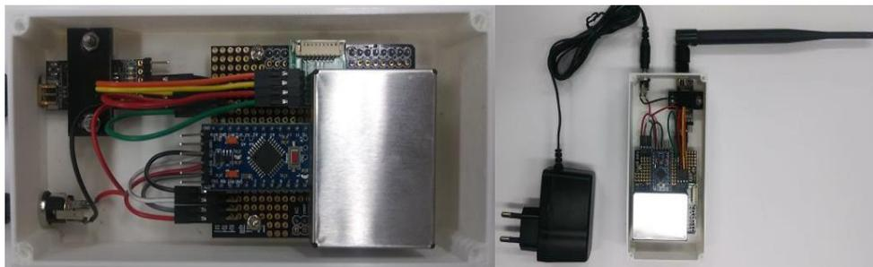
Fig. 10. PM sensor in which the low power mode was implemented.
