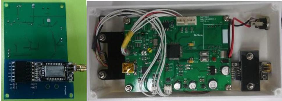
**Fig. 9.** The sensor board with an LPWA communication module applied, and the inside of the PM sensor module
