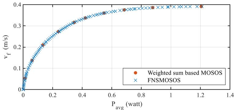
**Fig. 10.** Pareto optimal solutions obtained by FNSMOSOS and weighted sum based MOSOS
