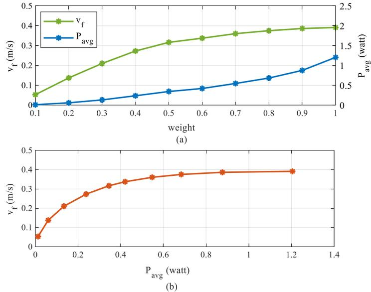
**Fig. 7.** (a) The effect of weight factor on the forward velocity and the average power consumption (b) Pareto optimal solutions
