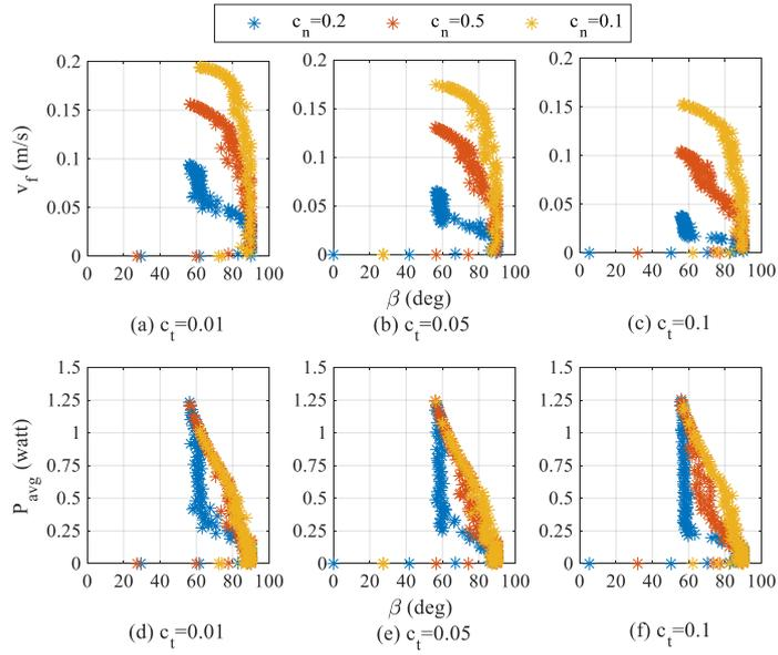
**Fig. 14.** The effect of different friction coefficients acting in the direction normal to snake robot on the forward velocity and average power consumption according to the optimal  $\beta$  parameter
