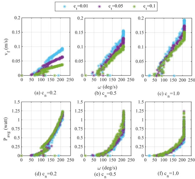
**Fig. 18.** The effect of different friction coefficients acting in the direction tangential to robot on the forward velocity and average power consumption according to the optimal  $\omega$  parameters
