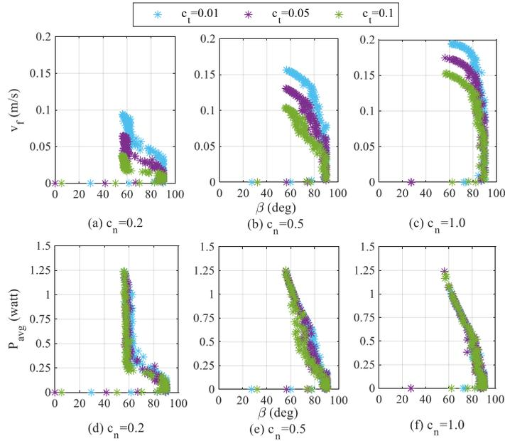
**Fig. 17.** The effect of different friction coefficients acting in the direction tangential to robot on the forward velocity and average power consumption according to the optimal  $\beta$  parameters
