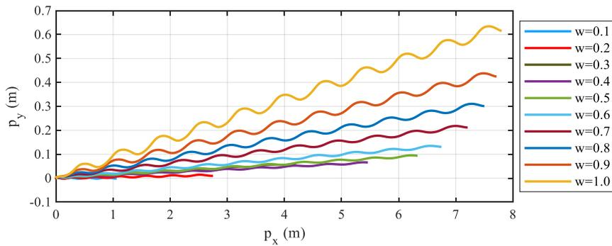
**Fig. 9.** The position of the CM of snake robot for each of the weight factor
