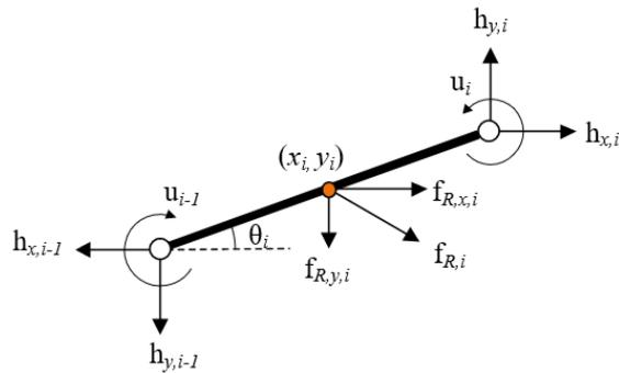
Fig. 2. The forces and torques acting on each link of the snake robot
