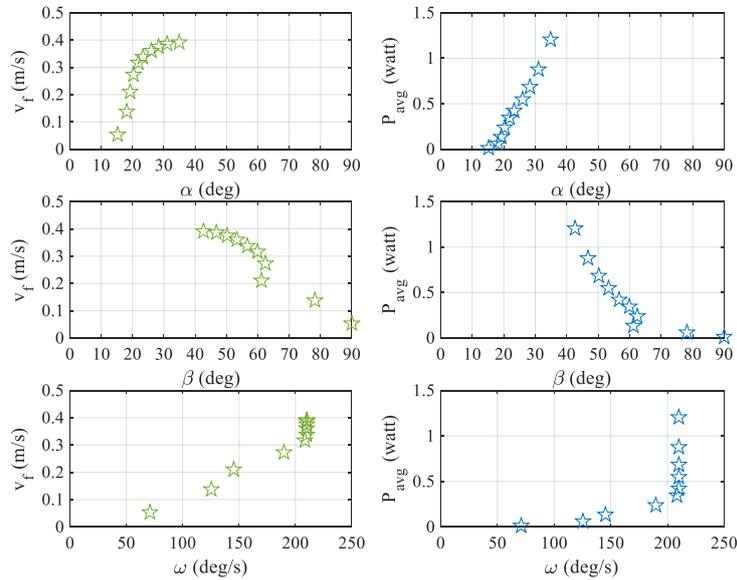
**Fig. 8.** The change of the forward velocity and the average power consumption versus optimal gait parameters
