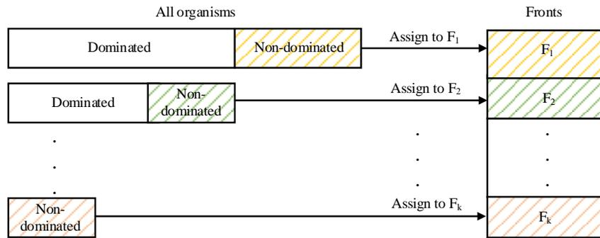
Fig. 5. A general scheme of non-dominated sorting procedure
