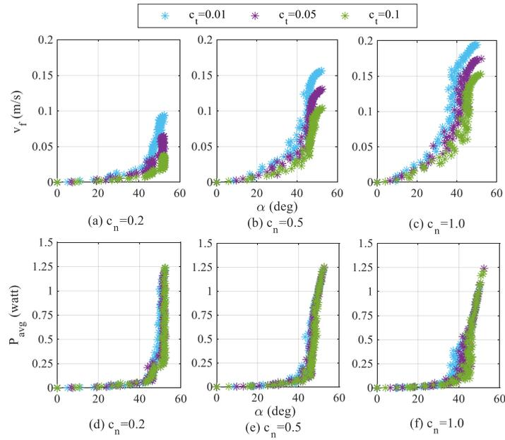
**Fig. 16.** The effect of different friction coefficients acting in the direction tangential to robot on the forward velocity and average power consumption according to the optimal  $\alpha$  parameter
