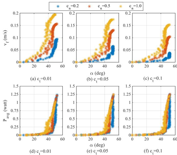
**Fig. 13.** The effect of different friction coefficients acting in the direction normal to snake robot on the forward velocity and average power consumption according to the optimal  $\alpha$  parameter
