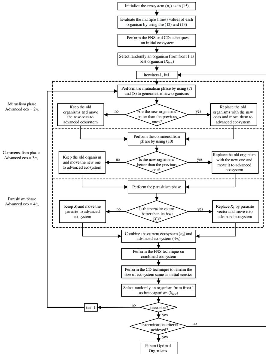
Fig. 4. The flowchart of proposed FNSMOSOS algorithm
