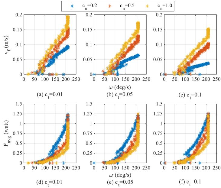
**Fig. 15.** The effect of different friction coefficients acting in the direction normal to snake robot on the forward velocity and average power consumption according to the optimal  $\omega$  parameter
