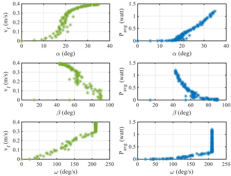
**Fig. 11.** The change of the forward velocity and the average power consumption versus Pareto optimal gait parameters
