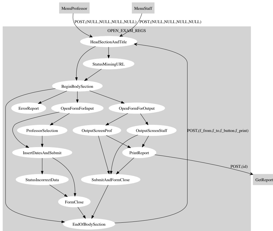
Fig. 7. The CIM for the dynamic page for processing open exam registrations.
