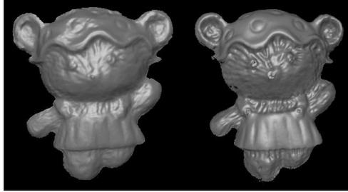
**Fig. 5.** The left Bear's shape was obtained using the traditional photometric algorithm, while the right shape was obtained using our extended algorithm
