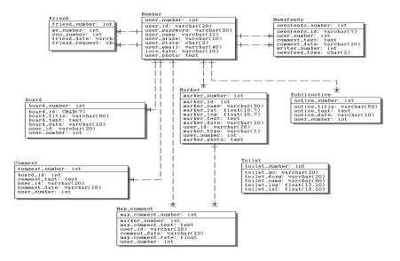
Fig. 7. A physical data model for the proposed system
