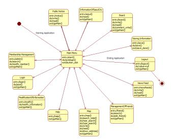
Fig. 8. The proposed state diagram
