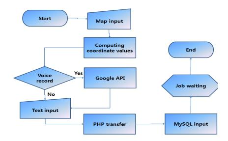
Fig. 11. A flowhchart for inserting coordinate values
